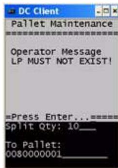
**Figure 28** Operator Message: Splits must be made to a new pallet
